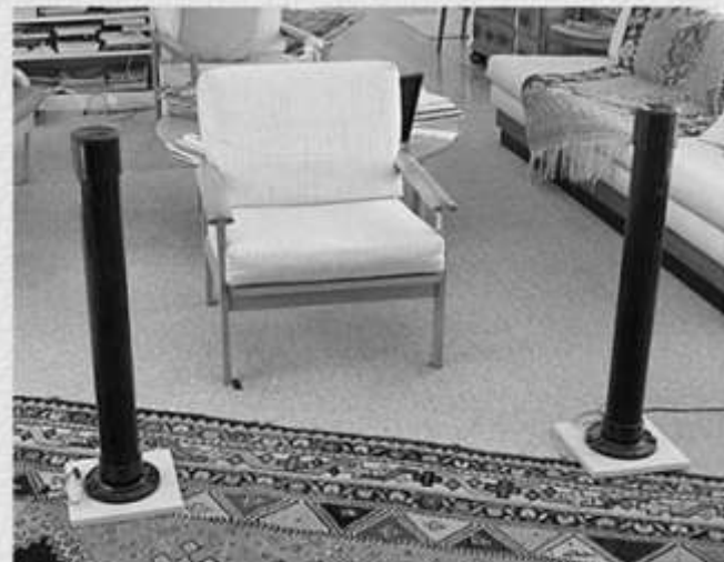
Figure 1: Loudspeaker setup in an equilateral triangle with the listener's head.
