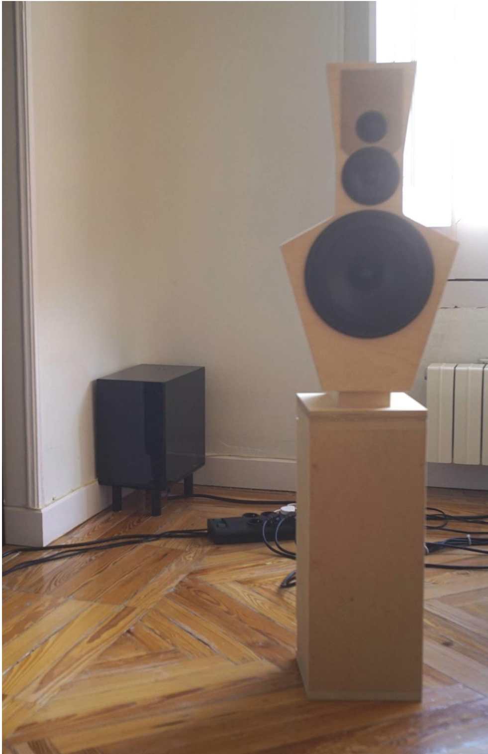
LX521 top on stand with dual 5" subwoofers in front corners
