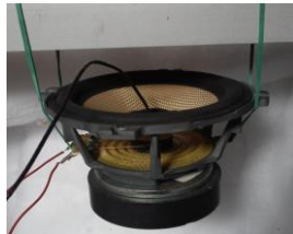
Figure 9: accelerometer mounted on the dust cap
