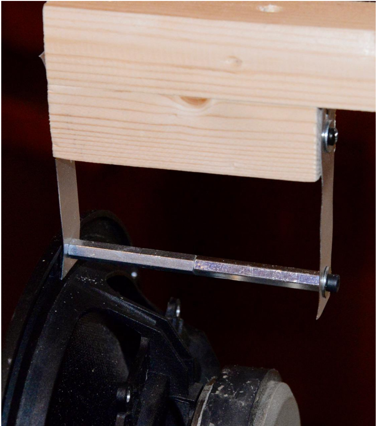
Close-up of the suspension system
