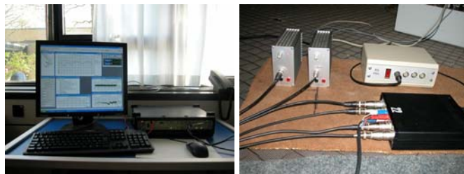
Figure 22 – The personal computer and the PULSE equipment used for measurement of the spectra (left); and the power amplifiers and active cross-over network with power supply, which were located within the anechoic room (right) .
