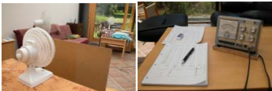
Figure 47 – A rear-view showing the other side of the set-up. The remote fan was not in use and the doors were shut to keep noise low. The measurement equipment consisted of a home-build instrument with preamplifier, third-octave filter and true RMS rectifier.
