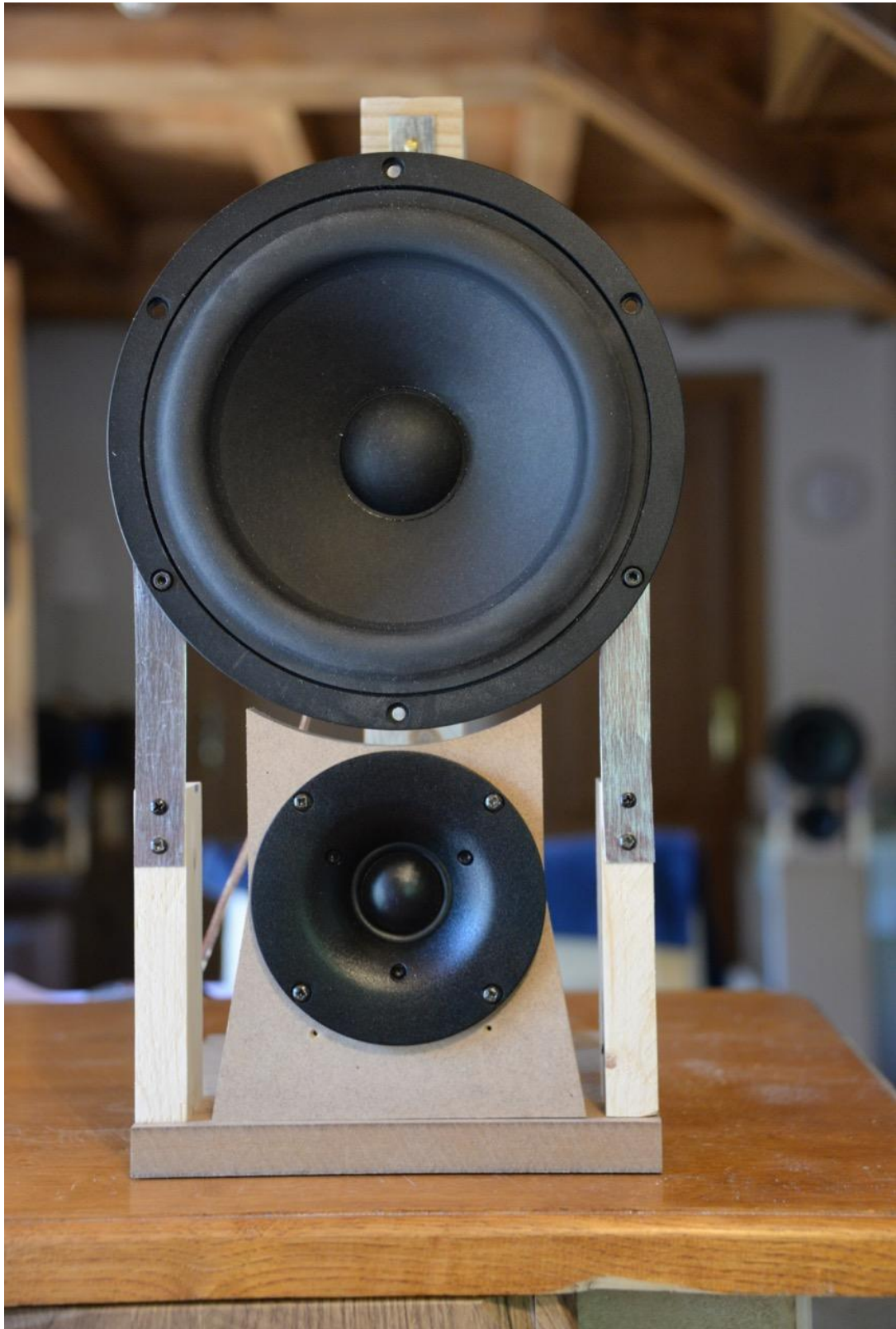
Main speaker with three leaf springs using Wavecor WF223BD02 and TW030A12
