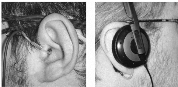
Figure 1 A recording and playback technique to generate identical sound signals at the eardrums. The same microphone tube next to the eardrum is used for recording and then to equalize the headphones.
