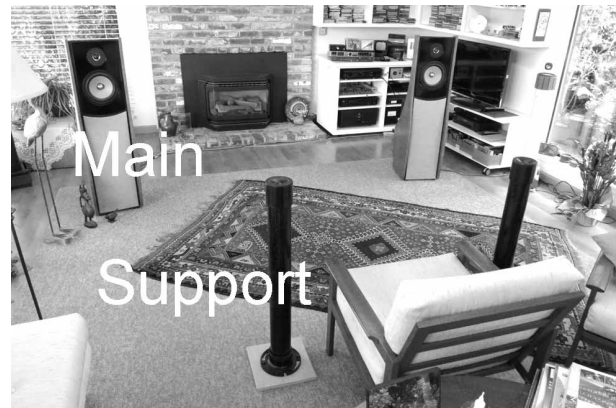
Figure 21 Stereo rendering with two acoustically small dipoles at standard distance and two omni-directional loudspeakers covering the ITD frequency range in close proximity to the listener
