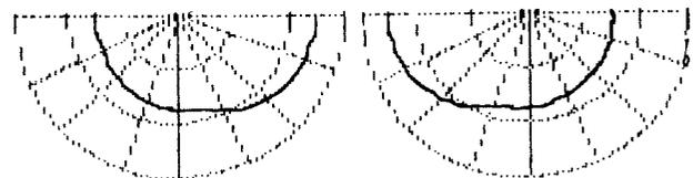
Fig. 2. Radiation pattern for well-fused off-centerline imaging. Maximum amplitude difference 9–10 dB for two conventional two-way loudspeakers less than 10 ft (3 m) apart (10 dB/div).
