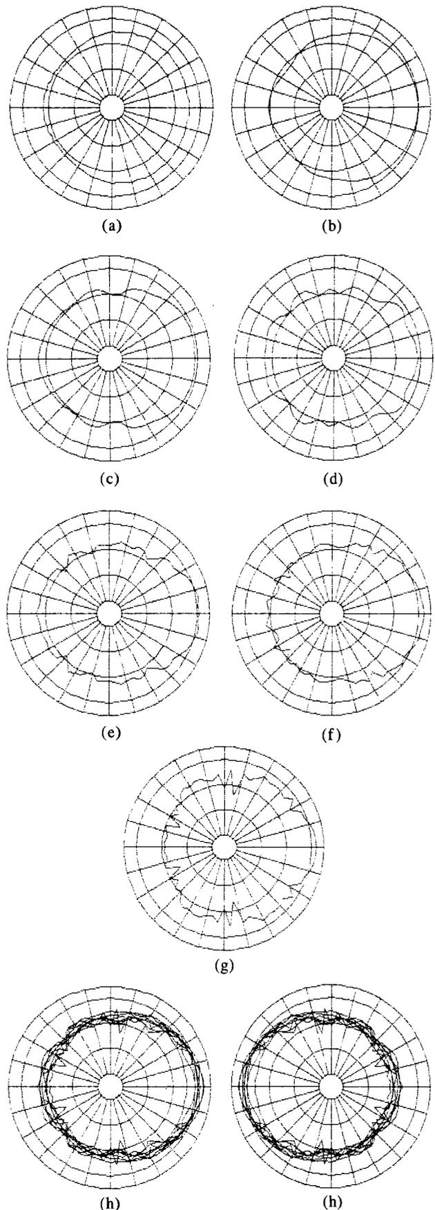
Fig. 11. Horizontal radiation for 14-driver equalized loudspeaker system, bundled by octave. 10 dB/div, left loudspeaker only shown. (a) 175–350 Hz. (b) 350–700 Hz. (c) 700 Hz–1.4 kHz. (d) 1.4–2.8 kHz. (e) 2.8–5.6 kHz. (f) 5.6–11.2 kHz. (g) 11.2–22.4 kHz. (h) Composite radiation pattern (stereo pair).
