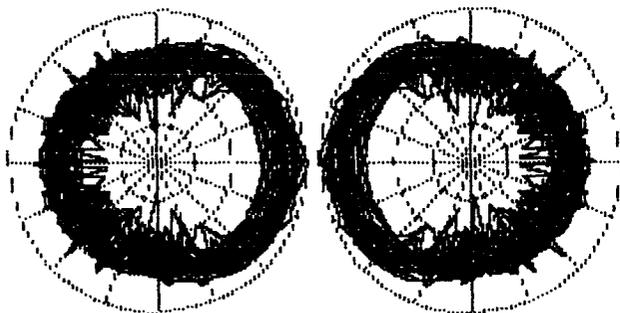
Fig. 7. Calculated horizontal radiation pattern for constant-imaging loudspeaker pair. Discrete frequencies, no averaging.
