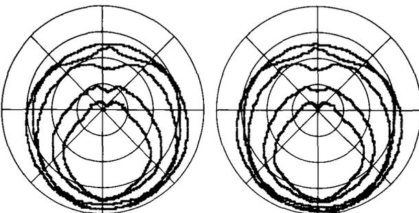
Fig. 5. Measured horizontal radiation pattern for conventional (forward-facing) multiway loudspeaker pair. Octaves, 20 Hz to 20 kHz.
