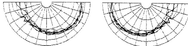
Fig. 14. Composite horizontal-radiation pattern for 5-driver loudspeaker system (stereo pair), bundled by octave. 10 dB/div, 175 Hz to 22 kHz. Front wall, 1 ft (0.3 m) behind loudspeakers, is included.
