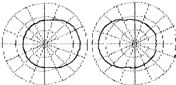
Fig. 3. Desired complete horizontal radiation pattern, after Fig. 2.
