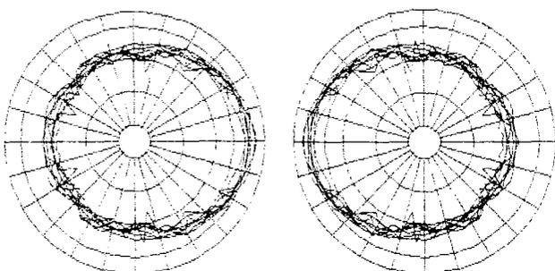
Fig. 8. Measured horizontal radiation pattern for constant-imaging loudspeaker pair. One-third octaves, bundled into octaves 20 Hz to 20 kHz.
