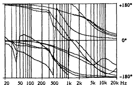
Fig. 10. Phase transfer function from input terminals to each of the drivers. 180°/div, 20 Hz to 20 kHz.
