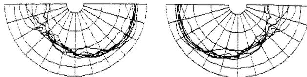
Fig. 13. Composite horizontal-radiation pattern for 6-driver loudspeaker system (stereo pair), bundled by octave. 10 dB/div, 175 Hz to 22 kHz. Front wall, 1 ft (0.3 m) behind loudspeakers, is included.
