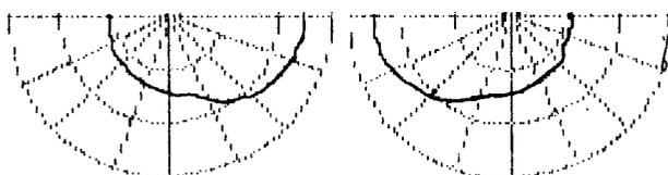
Fig. 1. Radiation pattern for well-fused off-centerline imaging. Maximum amplitude difference 14 dB, experimentally derived using two conventional two-way loudspeakers 10 ft (3 m) apart (10 dB/div).
