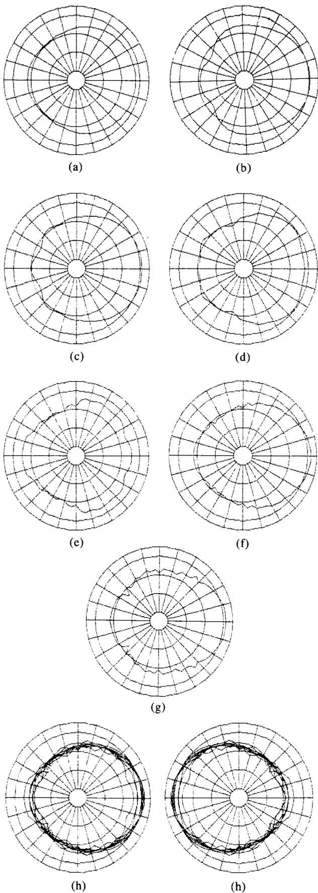
Fig. 12. Horizontal radiation for 8-driver equalized loudspeaker system, bundled by octave. 10 dB/div, left loudspeaker only shown. (a) 175-350 Hz. (b) 350-700 Hz. (c) 700 Hz - 1.4 kHz. (d) 1.4-2.8 kHz. (e) 2.8-5.6 kHz. (f) 5.6-11.2 kHz. (g) 11.2-22.4 kHz. (h) Composite radiation pattern (stereo pair).
