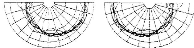
Fig. 15. Composite horizontal-radiation pattern for 4-driver loudspeaker system (stereo pair), bundled by octave. 10 dB/div, 175 Hz to 22 kHz. Front wall, 1 ft (0.3 m) behind loudspeakers, is included.
