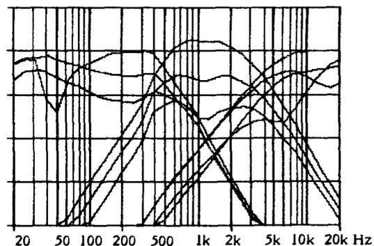
Fig. 9. Magnitude transfer function from input terminals to each of the drivers. 10 dB/div, 20 Hz to 20 kHz.
