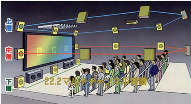
Fig 1: NHK (Hamasaki) 22.2 loudspeaker setup, as broadcasted by Japanese ARIB from 2016 onwards.<sup>2</sup>
